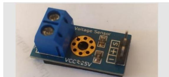
Gambar 10. Modul *voltage sensor*
